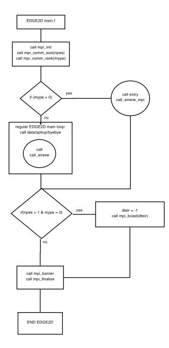
Figure 1: Flowchart of EDGE2D main routine with MPI support included. npes is the number of available cpu cores whereas mype is the rank (cpu core number) of the running process. EDGE2D is running on mype = 0 whereas all other cpus with mype > 0 are in wait-state until EIRENE is actually called. dteir normally defines the current EIRENE time-step (or zero when run in time-independent mode) but here dteir < 0 tells the main-routine to finalize and quit the program.
