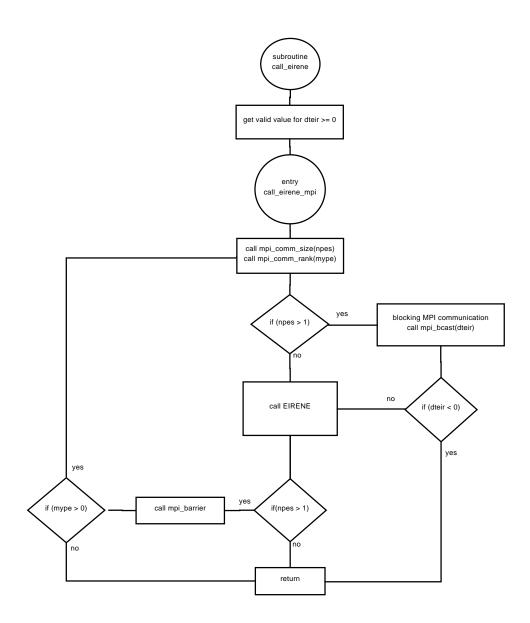
Figure 2: Flowchart of EIRENE driver routine called by EDGE2D with MPI support included. Definitions for mype, npes and dteir as in fig. 1. All cpus are active until EIRENE exits successfully. Cpus with mype > 0 are idling as long as the outer EDGE2D main-routine is executed.
